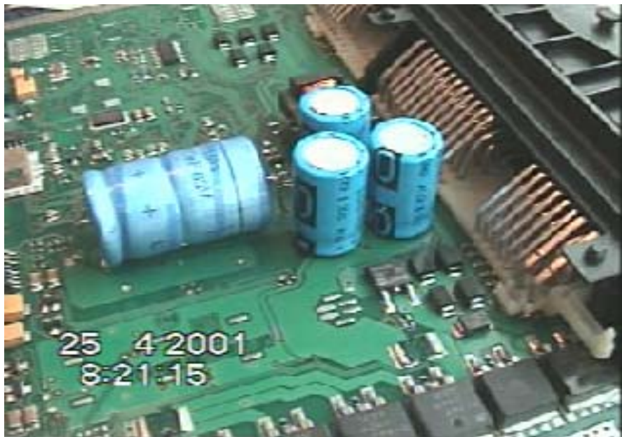
Figure 10 Electrolytic capacitors in a motor vehicle injection circuit from Bosch
